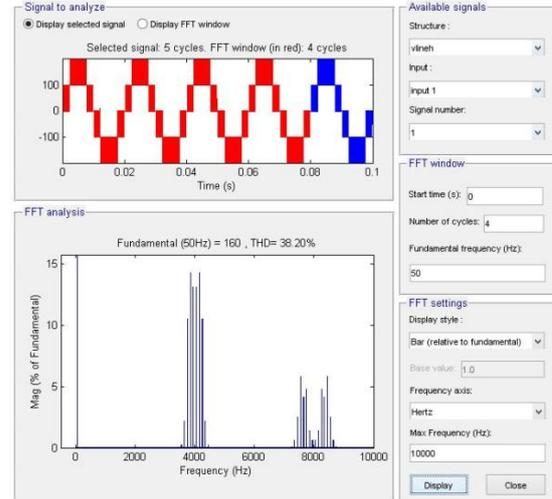
Fig. 8: Harmonic spectrum for phase voltage.
