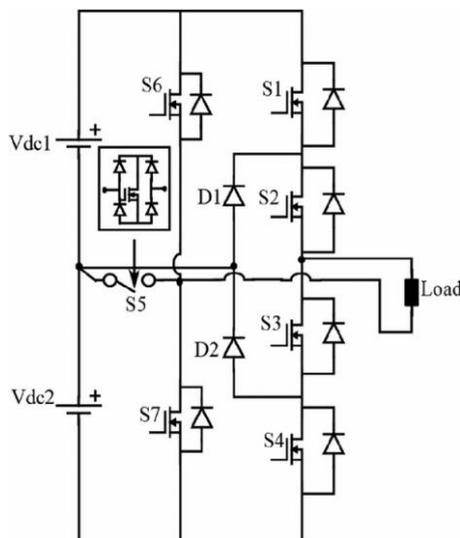
Fig. 2. Proposed fault-tolerant single-phase five-level inverter.
