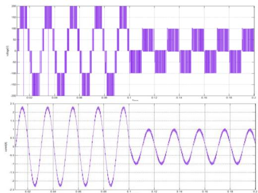
Fig. 6. Output voltage and current waveforms of the proposed inverter due to Vdc2 source failure (Y -axis 200 V/div, 2 A/div; X-axis 20 ms/div)
