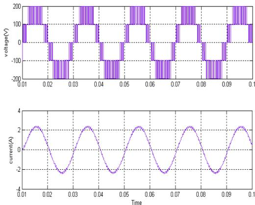
Fig. 5. Output voltage (upper trace) and current (bottom trace) waveforms of the five-level inverter (Y -axis 200 V/div, 2 A/div; X-axis 10 ms/div).
