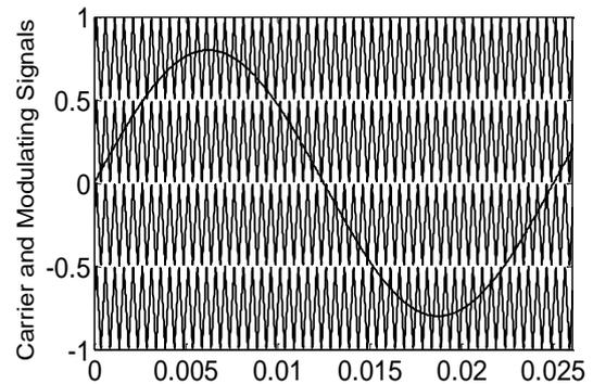
Fig. 4: Modulating and carrier waves for generating pulses in SPWM.
